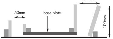
Cross Section of typical grouting formwork
